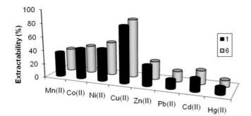
**Figure 4.** Extraction percentage of the metal picrates with ligands.  $(1 = H_2L^1, 6 = H_2L^2)$ ,  $H_2O/CHCl_3 = 10/10$  (*v/v*): [picric acid] =  $2 \times 10^{-5}$  M, [ligand] =  $1 \times 10^{-3}$  M, [metal nitrate] =  $1 \times 10^{-2}$  M, 298 K, 1 h contact time.
